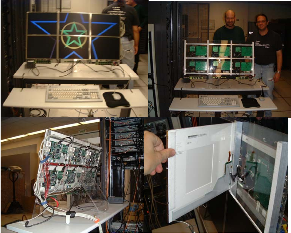
Figure 1: Images of the Personal Display Wall (PD-Wall). The upper left image shows the wall running the Distributed Memory Xserver (DMX) to create a single logical desktop from the multiple panels. The upper right image shows the simple aluminum and Plexiglas construction of the flatpanel. The lower left image shows the back of the display panel. The lower right image shows how the LCD's are affixed to the panel using Velcro – simplifying construction, assembly, and maintenance of the PD-Wall device. Each display of the PD-Wall is a single LCD laptop panel that can be purchased from an online vendor for about $200. The total cost of our prototype – a 3x2 array – was less than $1500, yet it provides an aggregate pixel resolution of 3072x1536.
